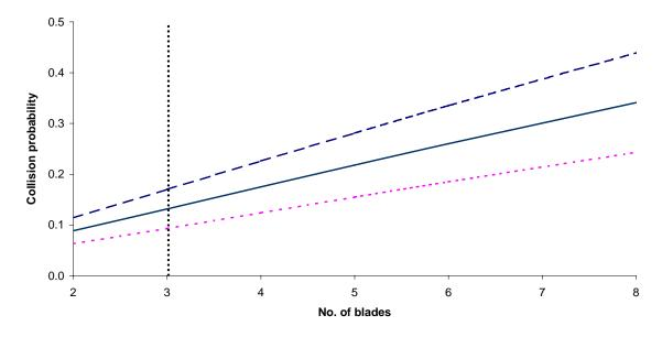
Figure 4 Effects on collision risk of variations in parameters used in the collision risk model (based on the SNHWB spreadsheet). The upper dashed line represents the 'upwind' scenario, the lower dotted line the 'downwind' scenario and the solid middle line the average between the two. In each case, original values (Fig. 1) remain constant apart from the parameter in question. Original parameter values are denoted by a vertical line.
